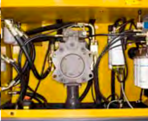
• Easy access to hydraulic pumps and filters.
