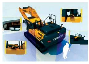
\* AAVM (All Around View Monitoring): Provides a field of vision in all directions with nine views including a 3D bird's eye view and a 2D/4CH view
