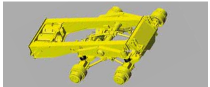
The Comfort-Ride option offers dual stage rubber blocks, which change the suspension characteristics to best match the laden and unladen haul cycles to maximise operator comfort.
